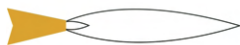
NEUTRAL FLAME (balanced oxygen and acetylene) For mild steel and general welding
